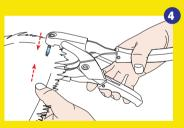
Before taking the sample, check that the cutter tip is present. Compress the tagger handles completely to take the sample.
